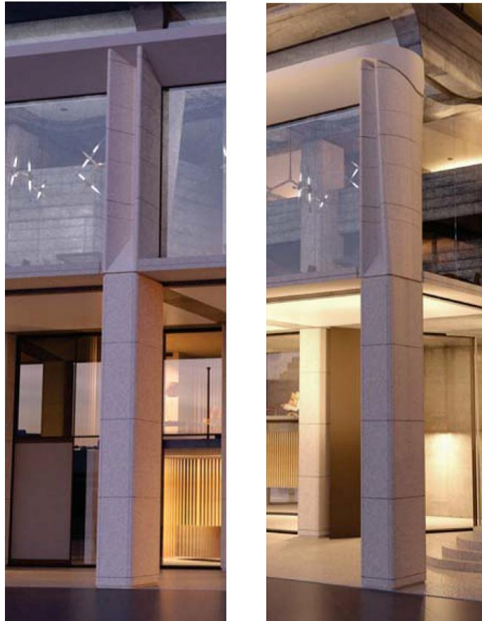
Figure 37: Photomontage of the proposed Images column design with rectilinear form at the bottom and twist at the top.
